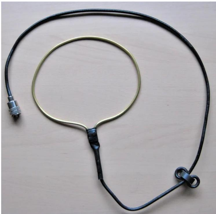
Messing, Rundstab, 4mm Durchmesser, Vollmaterial
