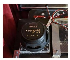
Connect the controller board to the SpeakerLightKit via the 3-pin connector and connect the system to the Pinball.
