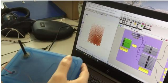
Figure 8. Example 2 is a facade simulation that allows user to 1) change the movement of sunlight by rotating the rotary potentiometer, 2) “open” and “close” facade by changing the density of the light sensor and 3) change color of facade by pressing the push button (Shen, 2019).
