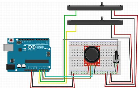
**Figure 12. Input device setup**
