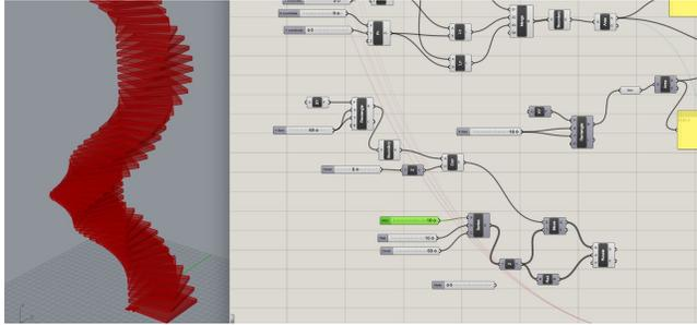
Figure 7. Example 1 is a simple simulation that allows users to 1) rotate geometry, 2) move geometry and 3) extrude geometry to a certain height (Shen, 2019).
