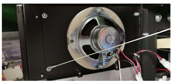
Connect the controller board to the SpeakerLightKit via the 3-pin connector and connect the system to the Pinball.
