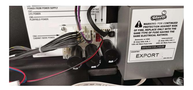
Place the voltage transformer (small black box) in the backbox and close the cover.
