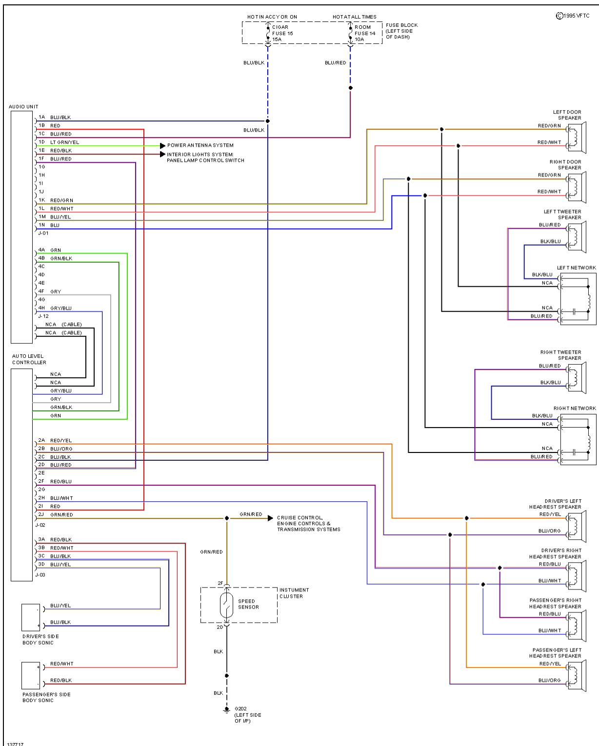
**Fig. 25: Premium Sound Radio Circuit**
