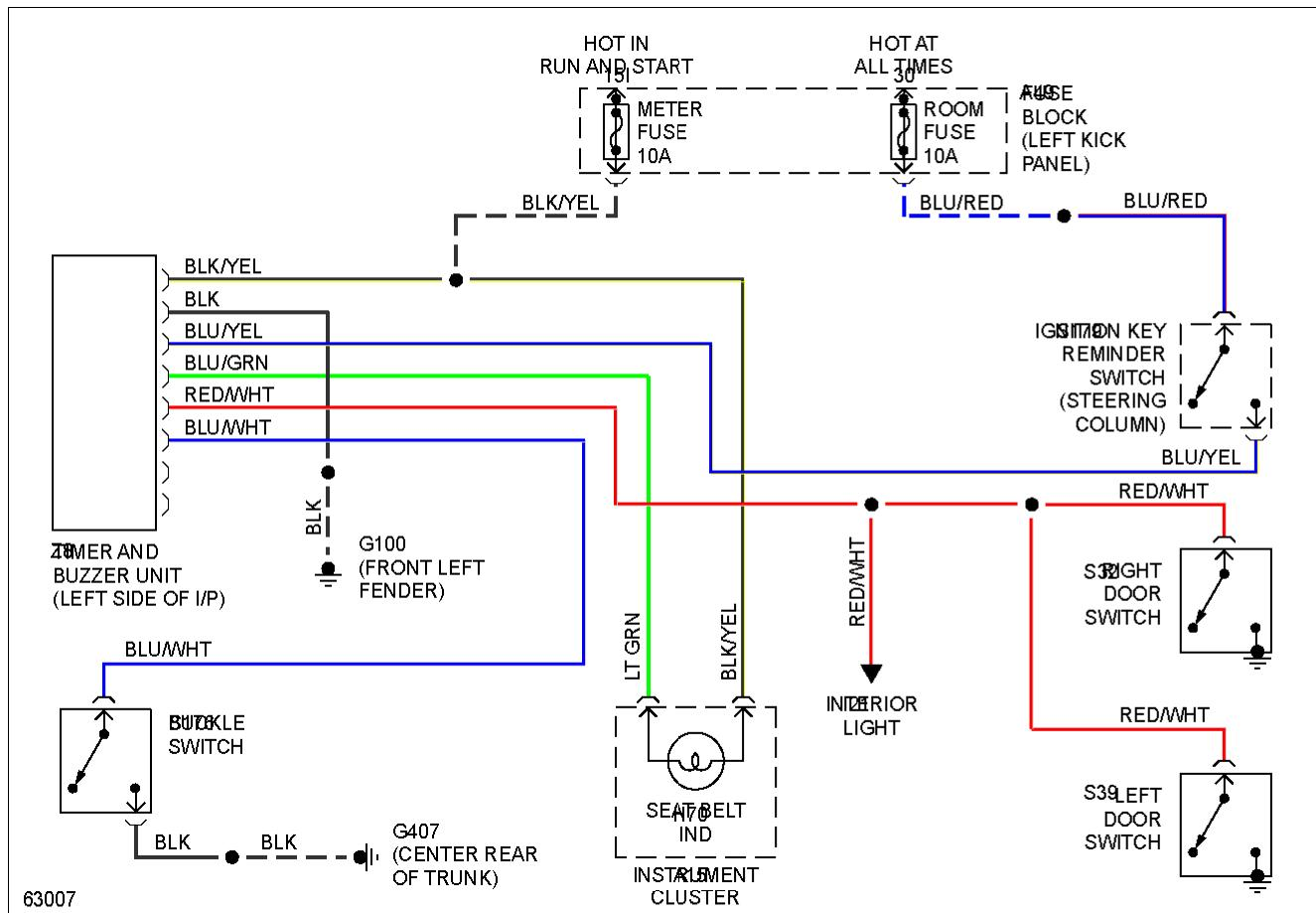
**Fig. 32: Warning System Circuits**
