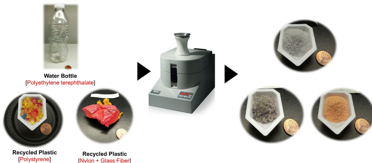
Fig. 1. Plastic samples were crushed using Fritsch Pulverisette-14.
