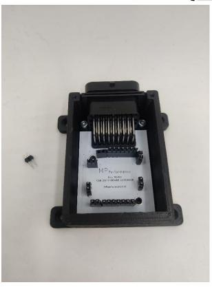
Step 3 Place the header pins in the Ecumaster CAN switchboard as shown in the picture
