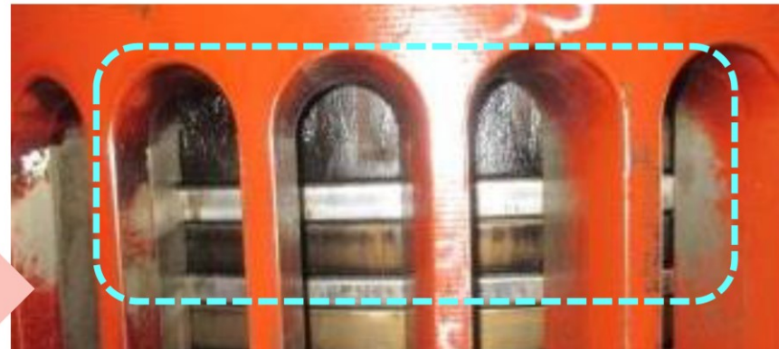
VLSFO + BN70 cylinder LO (Black deposit on piston-land has been reduced)
