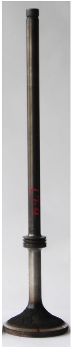
Valve spindle L7-4 Seating angle: 30°
