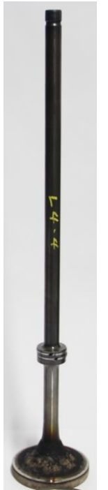
Valve spindle L4-4 Seating angle: 20°
