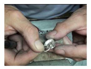
8. With the arm in position, mark through the tube hinge for the rivet hole. Drill through at this point and open the hole to fit the 1.6mm round wire off cut. It must be a tight fit. You can now put the components together whilst planning and marking for the catch opening. The catch will work most efficiently when it clicks into place at the top of the curved frame. You may need to bend the arm in a little to ensure it functions properly.
