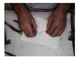
2. Use half round pliers to bend the strip of silver into the heart shape. When it comes to the point of the heart, cut squarely along the strip with your piercing saw before you bend it. This will make a sharper angle. Keep checking on your drawing to ensure it is symmetrical. Adjustments to the shape can be made easily if you overlap one end. Hard solder the connecting joint at the top and run solder into the mitre joint at the point.
