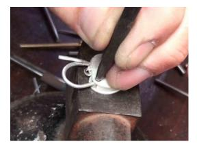
During the riveting process, keep checking that the arm still has free movement. Now push the arm into the body and ensure that the mechanism operates properly and clicks firmly in place. Cut several grip lines at the top of the arm. The arm should maintain springiness due to being core hardened. File the rivet ends flush with the body and emery clean the padlock before polishing.
