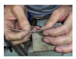
Drill out the excess wire from the tube. Tightly clamp the end of the wire into your vice. Grip the tube carefully with your draw tongs or similar and twist the wire around. Keep the wire taught and aim to twist it around two revolutions. This gives the wire maximum hardness as it is hardened right through its core as opposed to just surface hardening. This technique is ideal for catches & mechanisms.
