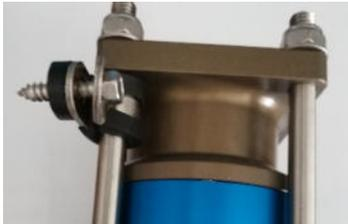
3. Press the Kärcher K2 high-pressure hose onto the valve mounted in the bottom right of the pipe cap. Secure the hose against slipping out with the two 2 mm rods. Once locked, bend the bars a little to prevent them from slipping out.
