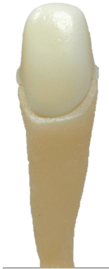
ZrO 2 cap after liner bake
