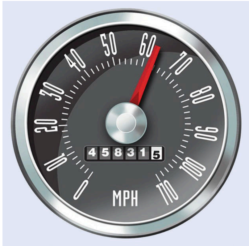
■ Fig. 16.10 Odometer from an automobile. The red arrow indicates speed, the numbers in the middle are the odometer that integrates that speedometer over time. The speedometer is the first derivative of the odometer. This is the essence of integral and differential calculus
