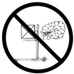
Never operate during high wind conditions. Lifting bulky loads during high winds can result in the lift tipping over and the possibility of operator injury.
