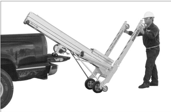
**IMPORTANT** Before tilting unit to reclined position, the carriage must be lowered all the way down and the Carriage Safety Latch must be engaged.
