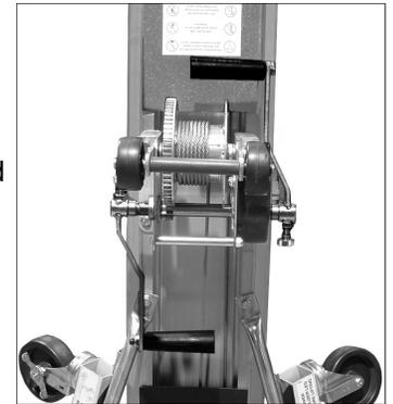
To place the winch handles in the operating position, pull up on the locking pin and slide the handle off of the winch shaft. Rotate the handle assembly around so that the black plastic grip is facing away from the winch. While pulling up on the locking pin, slide the handle back on to the winch shaft. Repeat this procedure for the other handle.
