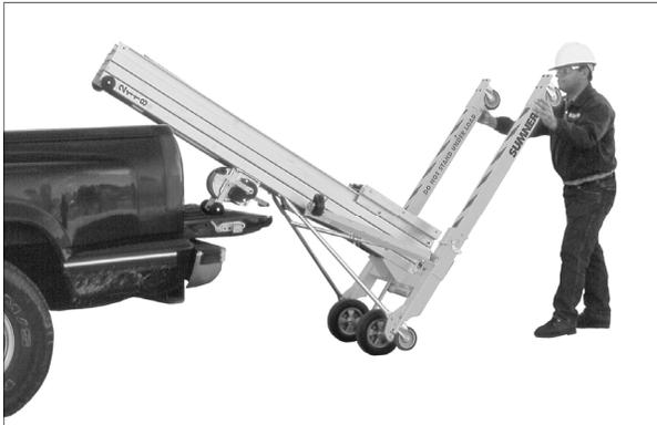
Unit may be loaded with a crane. Unit must be in upright and compact position with legs, forks, and stabilizers securely in their stored positions. If unit has any loose or unsecured items, remove them. Attach lifting hook to top roller bar located on top of bottom mast. Before elevating unit, lifting hook should always point away from the lift.
