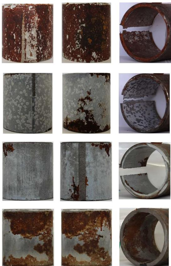
**Fig. 7.** Sealant/steel interface conditions. From top to bottom: Sealants S1, S2, S3, and S4.
