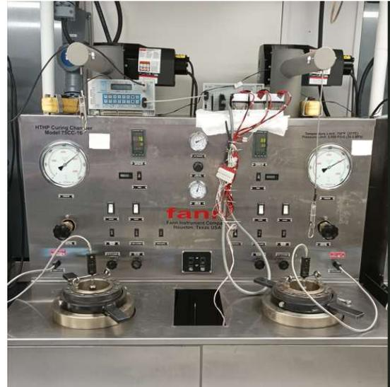
**Fig. 3.** Autoclaved chamber used for high temperature and high-pressure curing.
