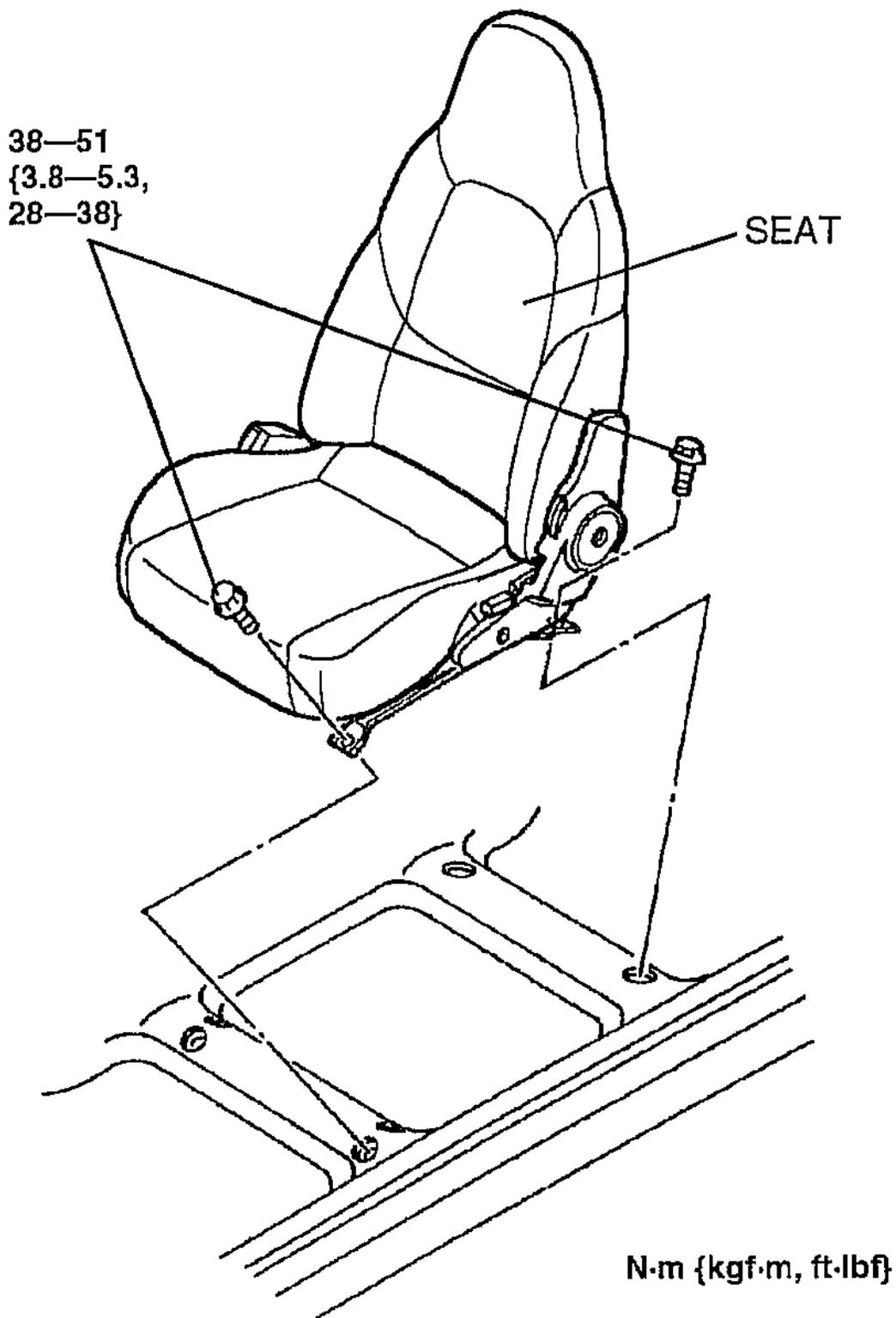
**Fig. 1: Removing Seat - With Torque Specifications**
