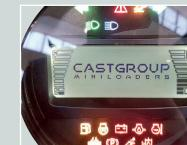
Electronic display with warning lights indicating faults, engine, hydraulic oil gauge, and electric floating system.
