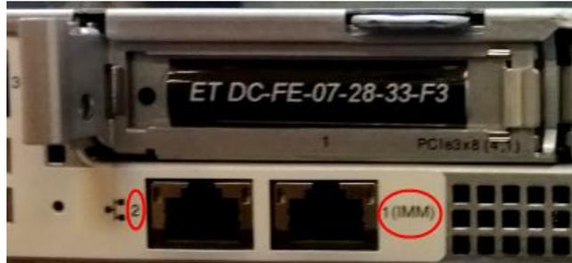
**Figure 9 Ethernet connectors in DocuSign SA Enterprise Hardware version 8.0 Back Panel**
