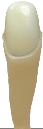
ZrO 2 cap after liner bake
