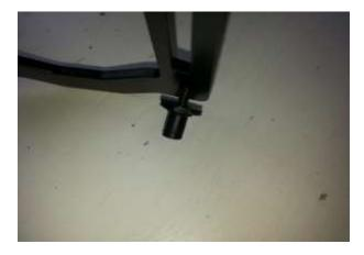
**3.** Pre-assemble the upper and lower adjuster brackets on the back side of the windscreen as seen in the picture below. Insert the hand knobs from the front side of the windscreen, steel and rubber washer positioned as pre-mounted on the hand knob. From the back side, first the 5mm spacer, then the adjuster bracket and finally the T-slot nut. Do not tighten the hand knobs, to allow for adjustment of the upper and lower parts.
