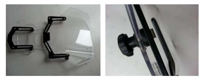
**4.** To mount the screen, start with the upper part. Slide the windscreen to the upper end of the adjustment, this way the two fastening holes are accessible. Place the M5x20 bolts through the two holes.
