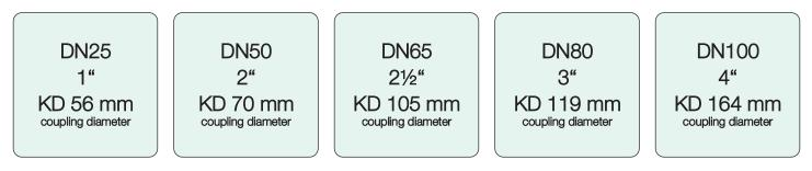
The coupling sizes 2" (KD70) to 4" (KD164) are manufactured in accordence with NATO STANAG 3756 and are compatible with other existing brands like DDCouplings® / TODO-MATIC® / Avery Hardoll®
