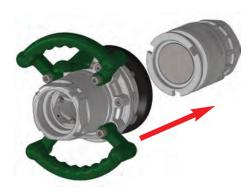
1. The coupler (hose unit) is pushed over the adaptor (tank unit) without canting until the three rollers - offset by 120° of the coupler have been completely guided through the slots of the adaptor. The position is not relevant.
