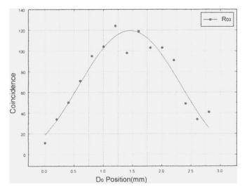
FIG. 5.  $R_{03}$  (joint detection rate between detectors  $D_0$  and  $D_3$ ) (Ref. 13).
