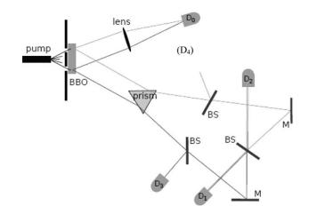
FIG. 2. Setup of the "quantum eraser" experiment of Kim et al. (Ref. 13).
