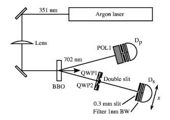
FIG. 8. Setup of the quantum eraser experiment of Walborn et al. (Ref. 14).
