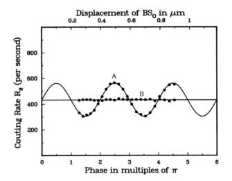
FIG. 7. Measured photon counting rate as a function of beam splitter  $BS_0$  displacement. Curve A: NDF between NL1 and NL2 (interference). Curve B: beam stop inserted between NL1 and NL2 (no interference) (Ref. 12).
