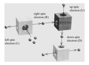
FIG. 15. If spin down or spin up electrons are routed again through a second horizontal box, we would expect that 100% spin right electrons are emerging from the horizontal box, but there result 50% spin right and 50% spin left electrons (Ref. 18).
