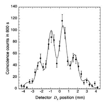
FIG. 12. Coincidence counts when QPW1, QWP2, and POL1 are in place. POL1 was set to  $\theta + \pi/2$ , the angle of the fast axis of QWP2. Interference has been restored in the antifringe pattern (Ref. 14).
