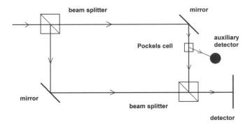
FIG. 1. Setup of the delayed-random-choice quantum mechanics experiment of Alley *et al.* (Ref. 10).
