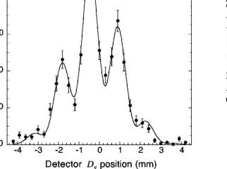
FIG. 9. Coincidence counts with QWP1 and QWP2 removed. An interference pattern due to the double slit is observed (Ref. 14).
