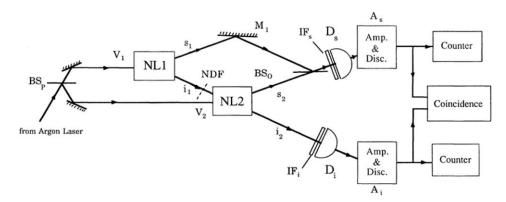
FIG. 6. Setup of the experiment of Mandel and coworkers (Ref. 12).
