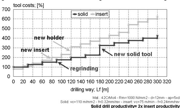
The requirement for this is a well-organized regrinding and recoating service. This secures quality and logistics, e.g. by outsourcing of the internal tool management.
