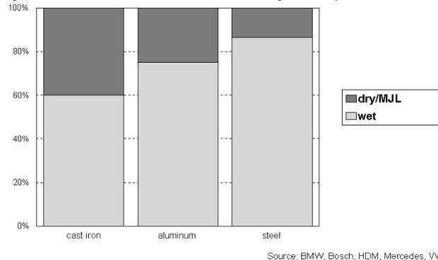
The expansion of dry machining can be greatly accelerated. A good example is this priority list of new investment guidelines already in use today by two large car manufacturers:
