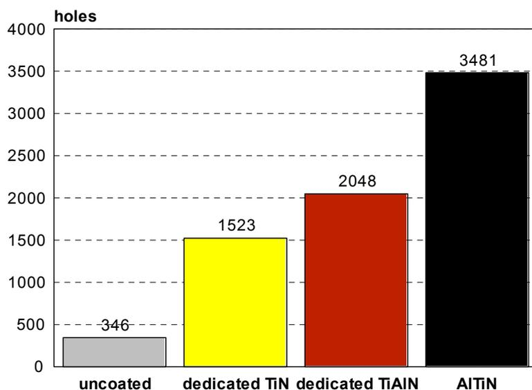
Tool: solid carbide drills - d=6.8mm - vc=80m/min - f=0.15mm/rev - ap=30mm
