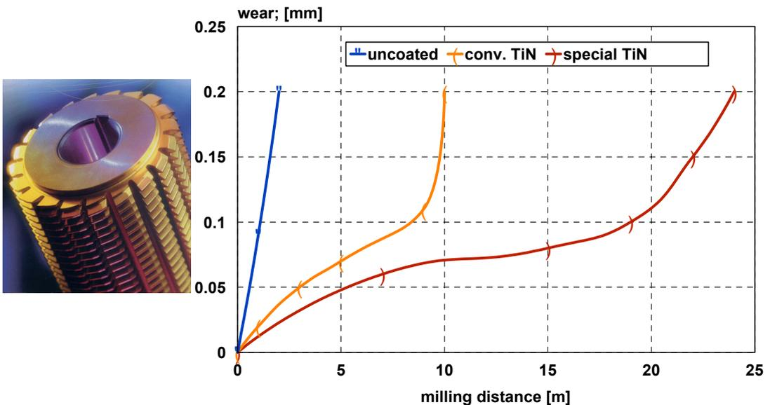
Mat.: 100Cr6 - Tools: ASP30 - d=80 x 180 mm - vc=135 m/min - coolant: emulsion
