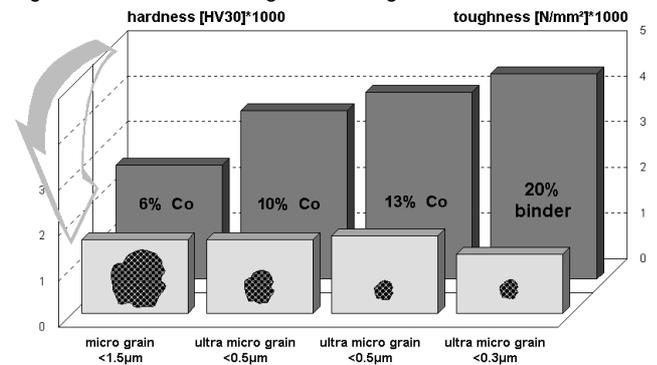
Highest toughness and hardness at the same time can be achieved today by using nanograin carbides. Because they are still exorbitantly expensive, carbides with a tough core and the hard surface using gradient structures are being developed (fig. 13).
