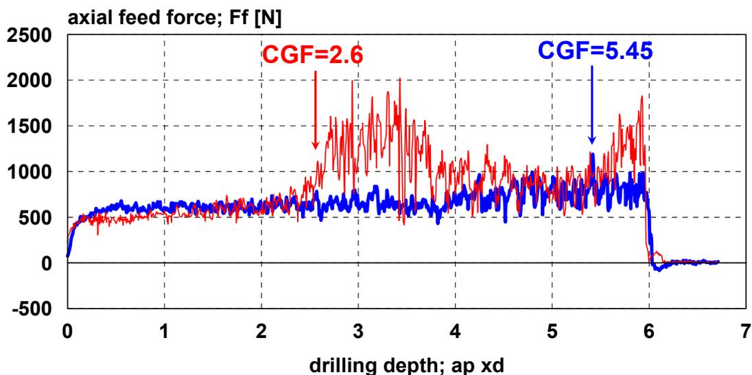
Mat.: GGG40 - Tool.: HSS-DIN 338 - d=6mm - ap=6xd - vc=30m/min - f=0.18mm/rev - dry
