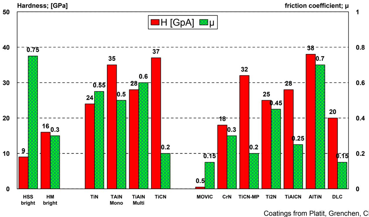
Not normally used for cutting, **CrN** is essential for forming tools and machine parts.
