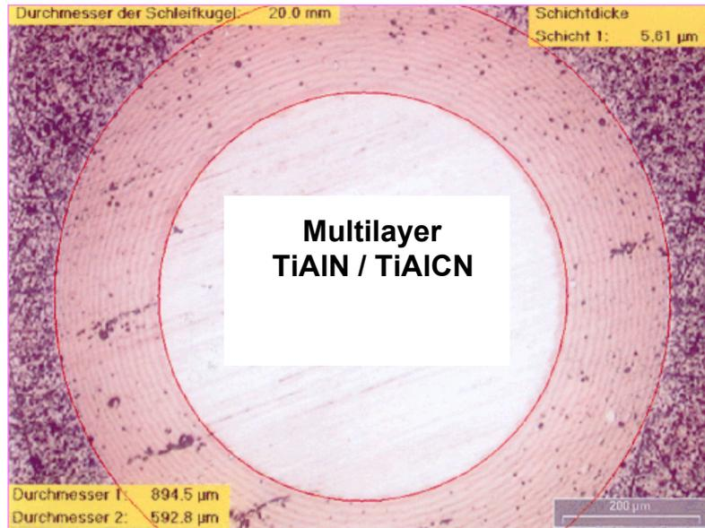
The multilayer structure achieves extremely good results even when compared to multilayers deposited in large coatings units.
