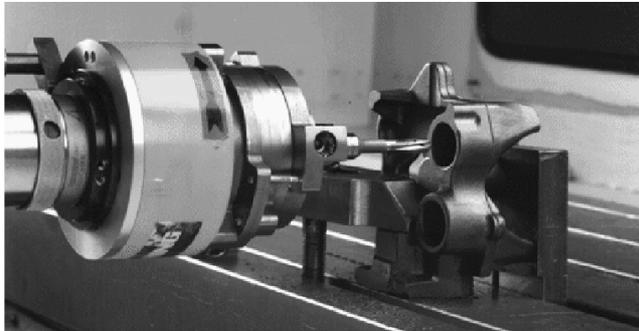
With all these advantages of minimal jet lubrication, are soft glide coatings still necessary? The answer is yes. Especially in "emergency situations", when the minimal lubrication can not, for whatever reason, reach the important parts of the tool. The author would like to dare to make the prediction that by 2005, the combination of minimal jet lubrication and soft glide coating will have replaced full coolant in up to 10% of all new German machining centers.
