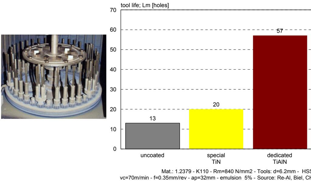
The increasing of the Al-content improves the heat resistance of the coating. Therefore the **AlTiN** coating with 67% Al is especially suitable for dry machining and for working with minimum lubrication.
