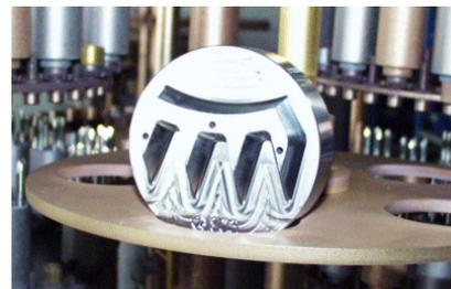
CrN can be coated at lower temperatures (~200 °C) as well and has at relatively high hardness a low friction coefficient.
