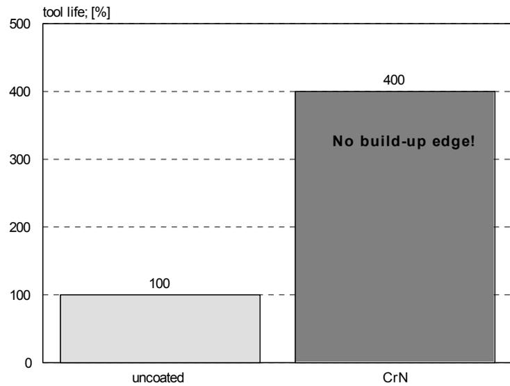
Mat.: Copper - Tool Mat.: tool steel - Coating temperature < 2
