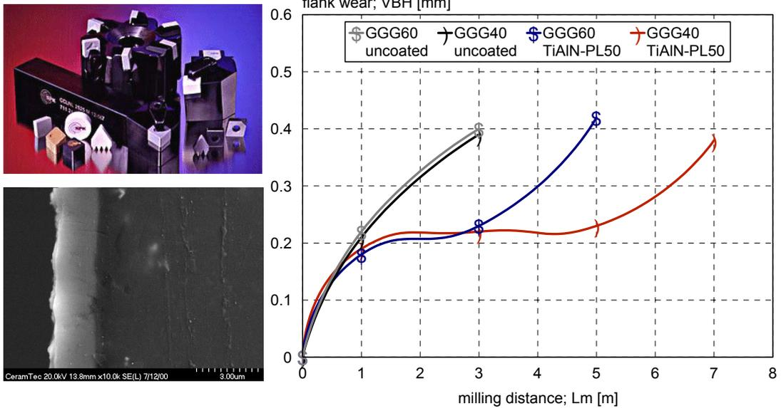
Tools: Silicon nitride ceramics inserts - SLC250C -  $v_c=400\text{m/min}$  -  $f=0.16\text{ mm/tooth}$  -  $a_p=2\text{mm}$
