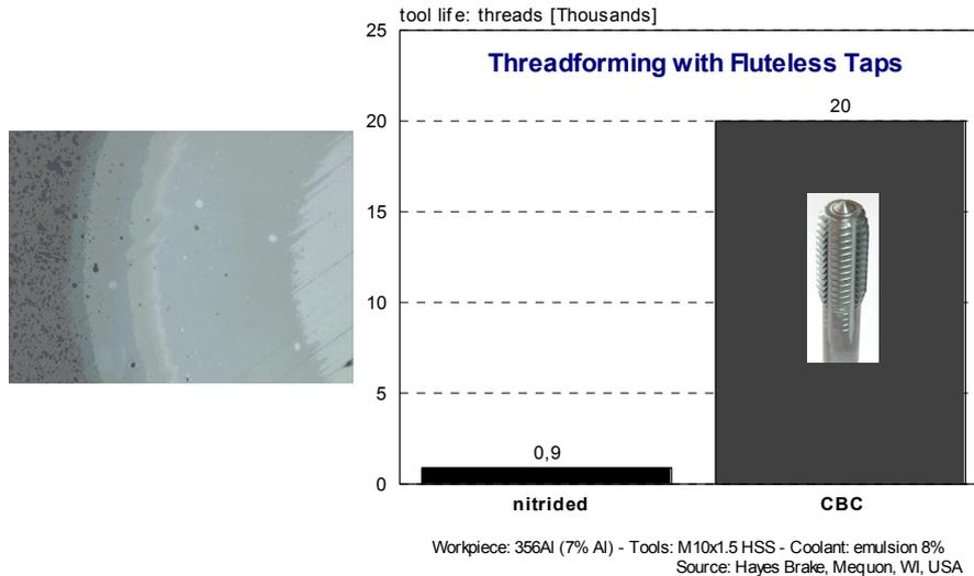
At working in harder materials the wear resistance will become important too. For these cases the combination of hard and lubrication coatings can be the solution.
