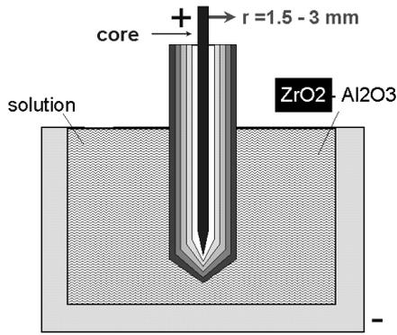
EPD-Gradient-Ceramic - ZrO<sub>2</sub> → Al<sub>2</sub>O<sub>3</sub>
