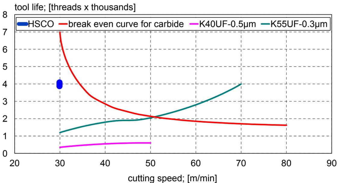
Mat.: C45 - connecting rod - Tool: M8 - ap=2xd - TiN- coolant: emulsion
