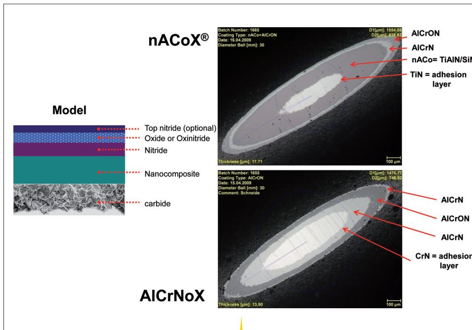
*Image 6: Structures of Oxide- and Oxynitride-Coatings from PLATIT.*
