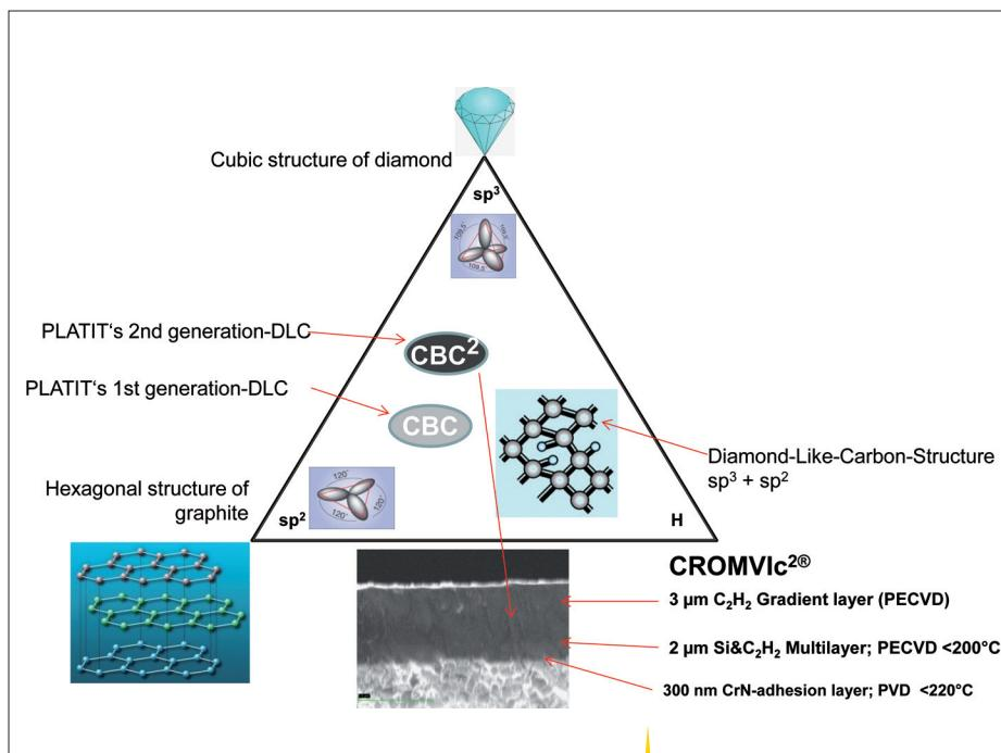
As a metal nitride basis is needed to prevent cracking and plastic deformation the coatings are (like with CVD) being built into a multi-layer structure (*image 6*).
