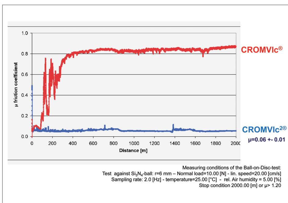
*Image 8: Comparison of Friction Behavior of PLATIT-DLC-Coatings.*
