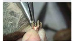
The claw tips can now be trimmed down and shaped with a needle file. Ensure the file has a safety edge to limit stone damage.
