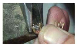
Jewellers generally need to make specialised tools for certain tasks. For the final forming of the claw tips, use a steel pusher with a 'V' shape cut into the end. This can be used to push and burnish the open edge of the tip until it closes fully onto the stone. It also hardens the tip for longevity.
