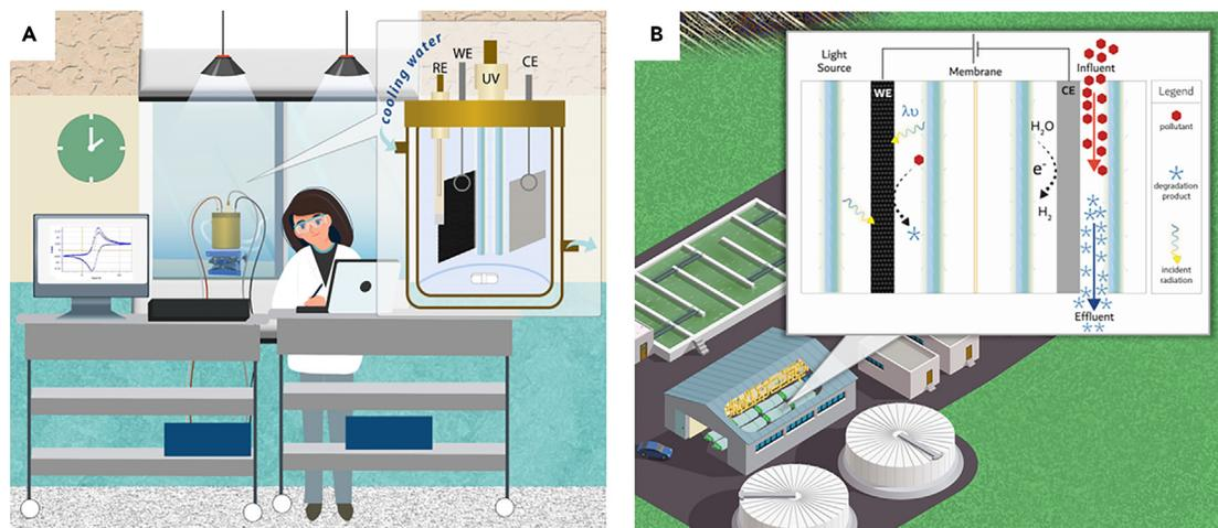
**Figure 1. Schematic illustrating photoelectrochemical systems**
