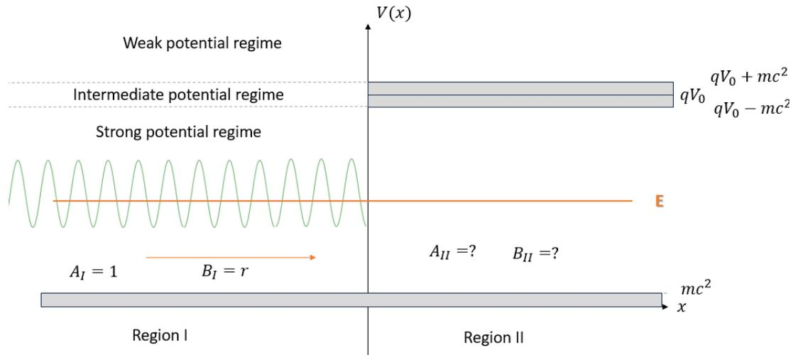
Figure 3.1: Particle scattering off the potential well of height  $qV_0$ ,  $V_0 > 0$ . The energy of the particle is positive and the particle is initially moving from left to right.
