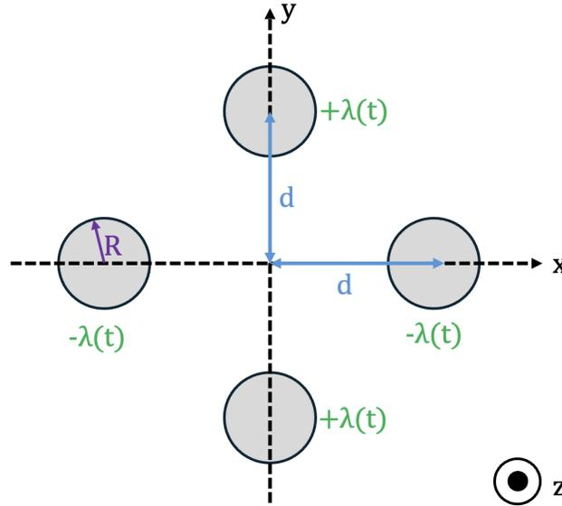
Figure 4.2: Four infinitely long electrically charged rods extending in  $z$ -direction with line charges  $\pm\lambda(t)$ .
