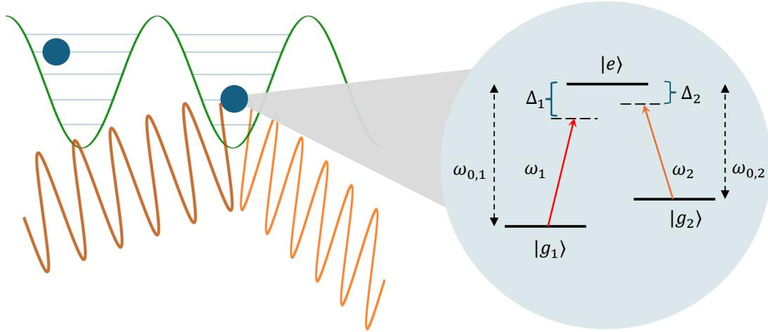
Figure 5.2: Illustration of standing wave potential for trapped atoms (left) and internal three level structure (right), with hyperfine ground states  $|g_1\rangle$ ,  $|g_2\rangle$  and excited state  $|e\rangle$ .
