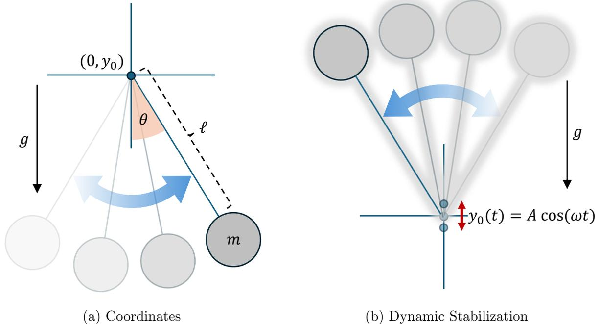
Figure 2.1: Definition of the coordinates for Kapitza's pendulum (a) and illustration of dynamical stabilization for a fast oscillating pivot point (b).
