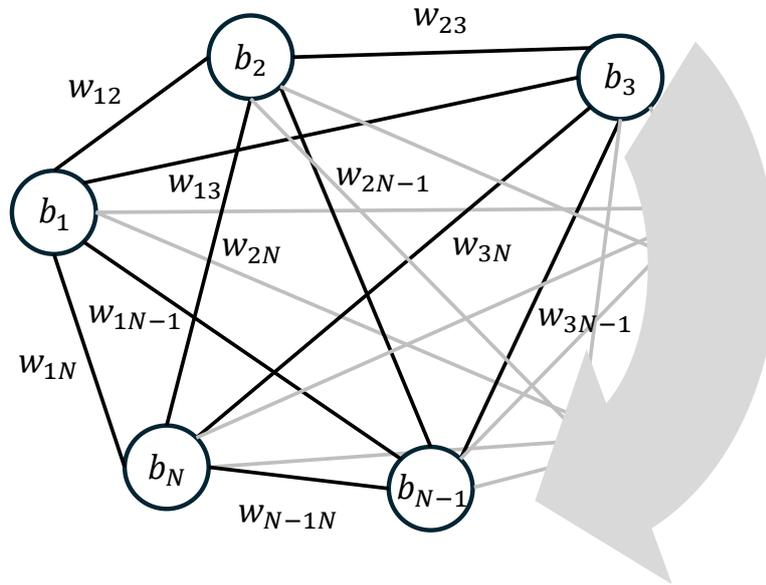
Figure 7.1: Illustration of a Boltzmann machine as an undirected graph, with edge weights  $w_{ij}$  and node weights  $b_i$ .
