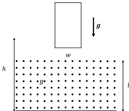
Figure 1.2: A conductor loop falling into a homogeneous magnetic field
