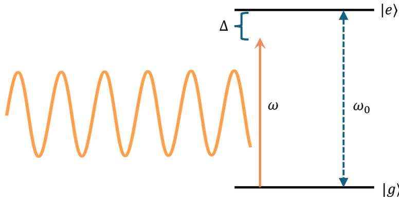
Figure 5.1: Two-Level system in an external field. Definition of variables and states.
