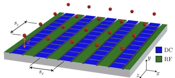
(b) Drawing of an ion trap chip from: P. Holz *et al.*, *Adv. Quantum Technol.* **3** (2020).
