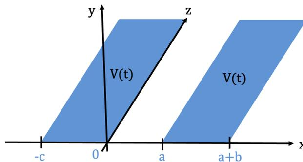
Figure 4.4: Two rf electrodes in the  $x, z$ -plane, with the rest of the plane grounded.
