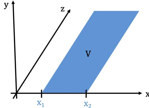
Figure 4.3: Electrode on voltage  $V$  extending in the  $x, z$ -plane, with the rest of the plane grounded.
