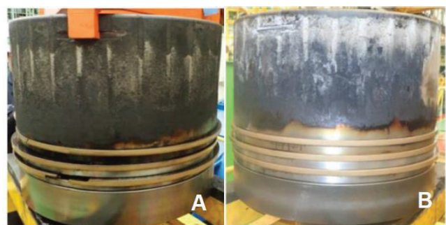
Figure 1: Example of condition after test bed. A. using a low-BN cylinder oil. B. using a 70BN cylinder oil.
