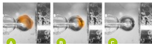
A contamination of the sensor B sonicclean active C clean sensor within 5 min*
