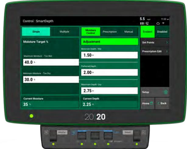
Figure 4. SmartDepth® Control System
