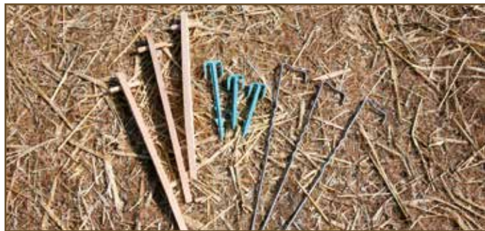
16.1 Variety of fixing pins to meet various soil conditions
