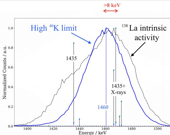
Figure 1: Monte-Carlo-Simulation with tRAYcy showing the intrinsic activity – the pure <sup>138</sup>La limit (spectrum = black dashed line, energy positions = black lines)–, versus the high <sup>40</sup>K limit (spectrum = blue line, energy position at 1460keV = blue).
