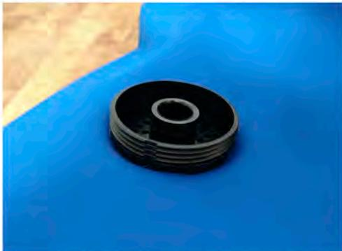
Put the body of the Boat Vent 3 into the hole. **NOTE:** Make sure the canvas is not covering the threads of the vent.
