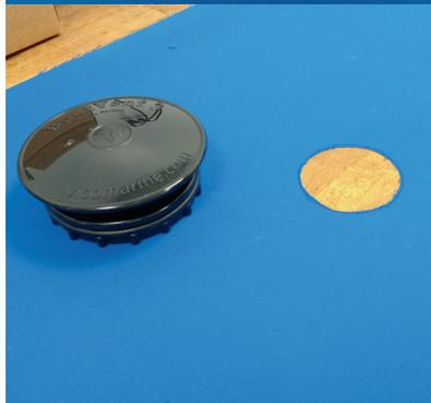
**5** Put the body of the Boat Vent 3 into the hole. **NOTE:** Make sure the canvas is not covering the threads of the vent.
