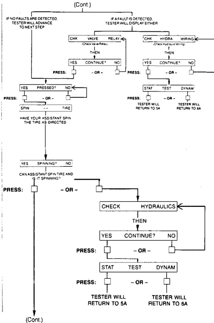
Fig. 24: 6C. Solenoid Test (2 of 4)
