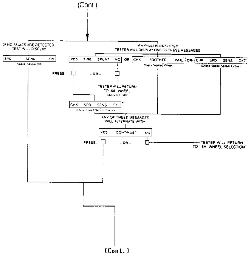
**Fig. 22: 6B. Dynamic Wheel Sensor Test (2 of 2)**
