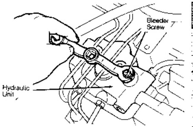
**Fig. 12: Locating Hydraulic Unit Bleeder Screw**
