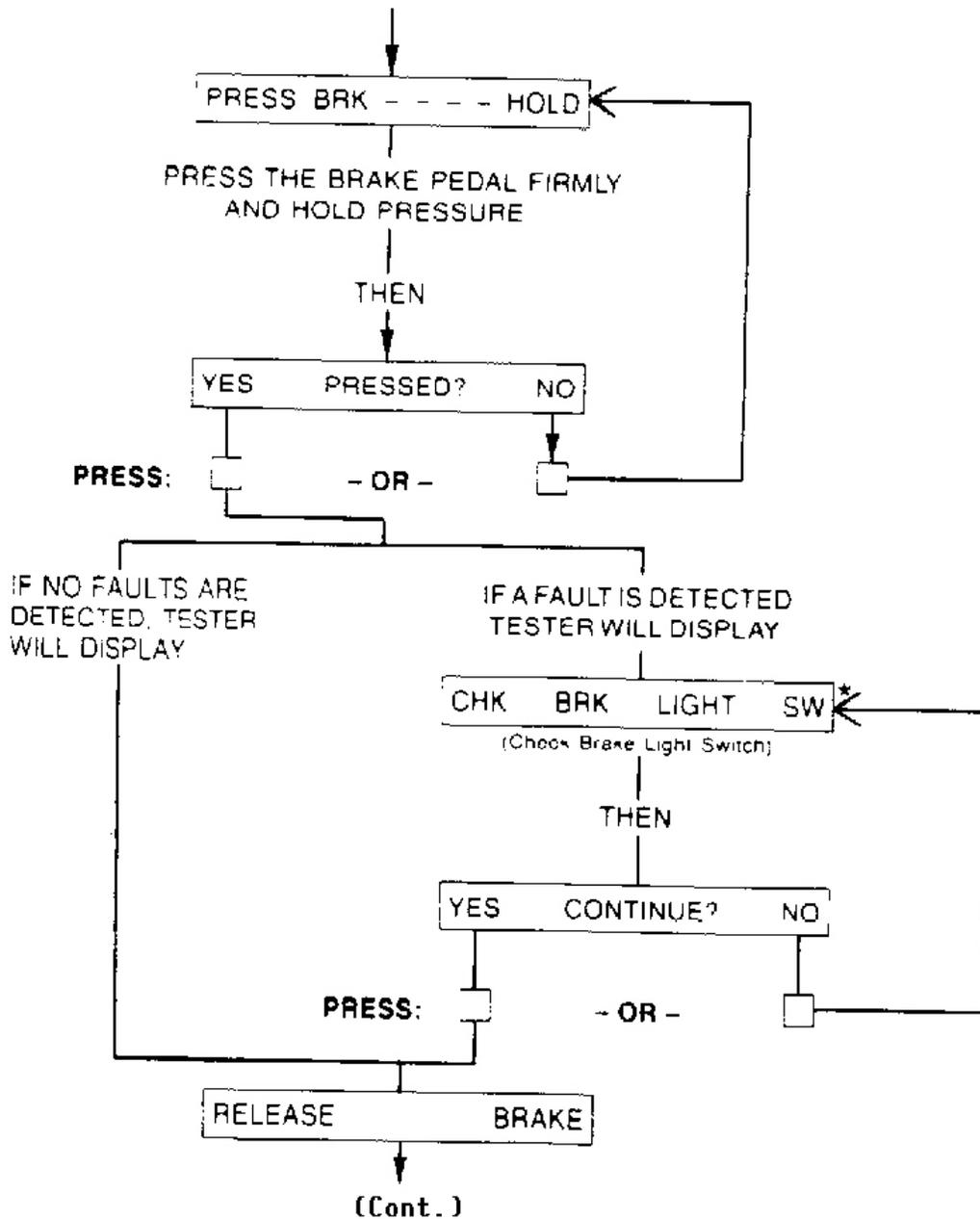
**Fig. 18: Test 5B. Brake Light Switch Test**
