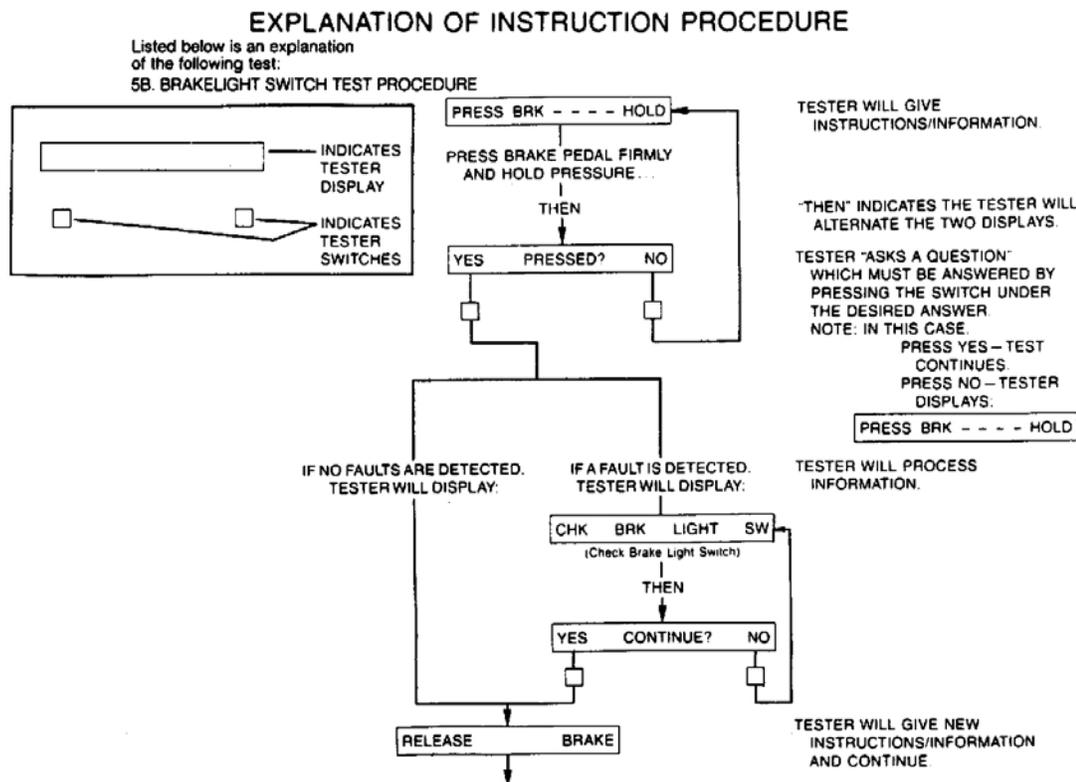
**Fig. 13: Operating ABS Tester**
