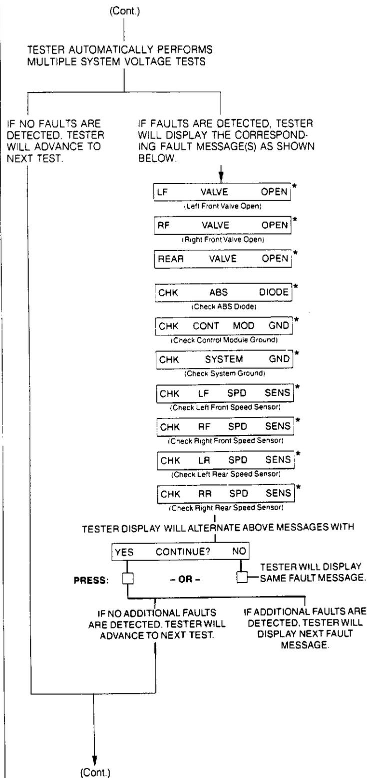
**Fig. 16: Test 4 System Voltage Test**
