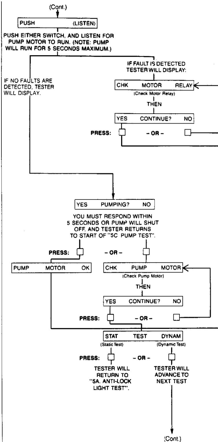
Fig. 19: Test 5C. Pump Test
