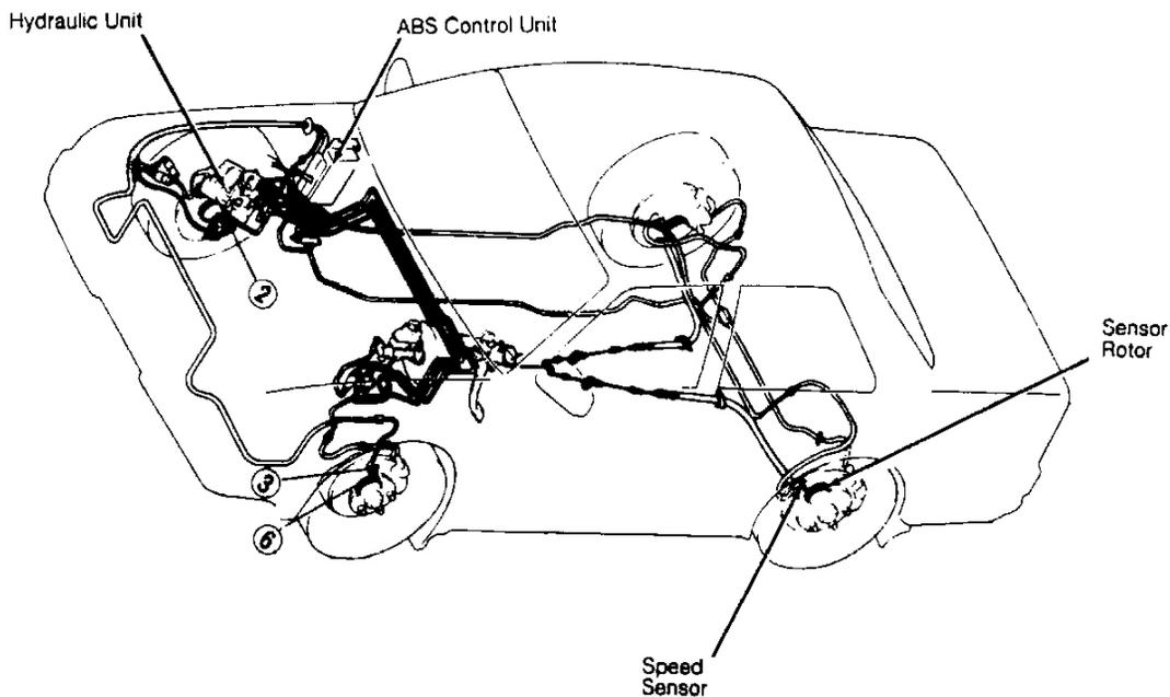
**Fig. 3: Locating ABS Components (929)**
