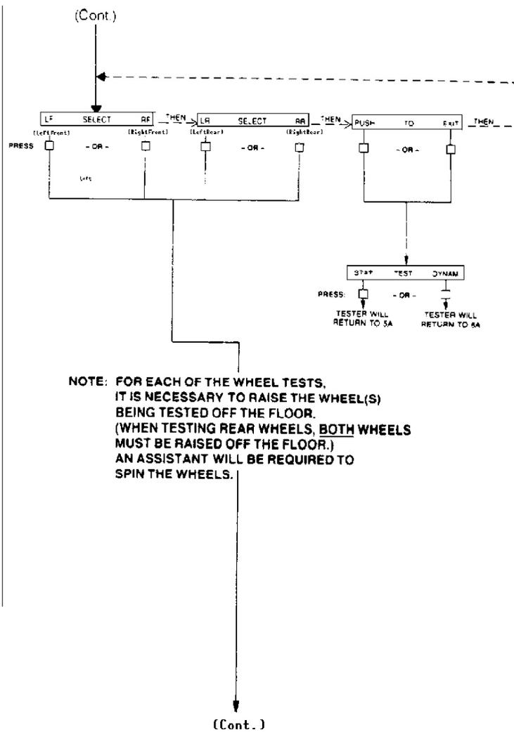
**Fig. 20: 6A. Dynamic Wheel Selection Test**
