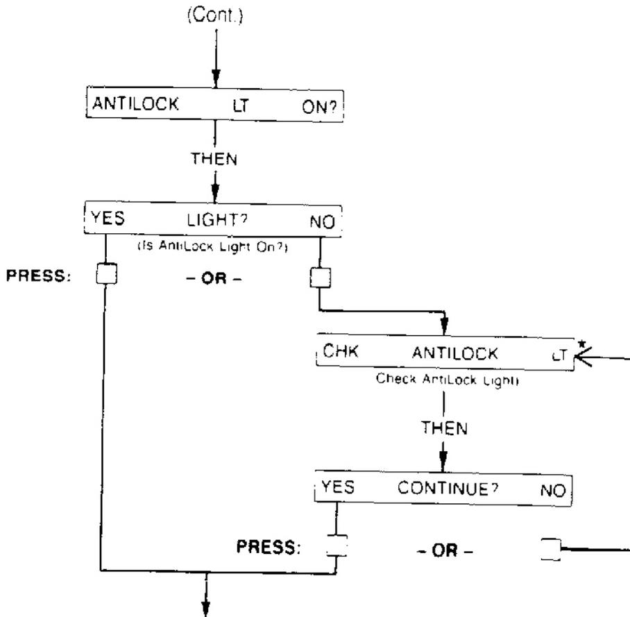
**Fig. 17: Test 5A. Anti-Lock Light Test**
