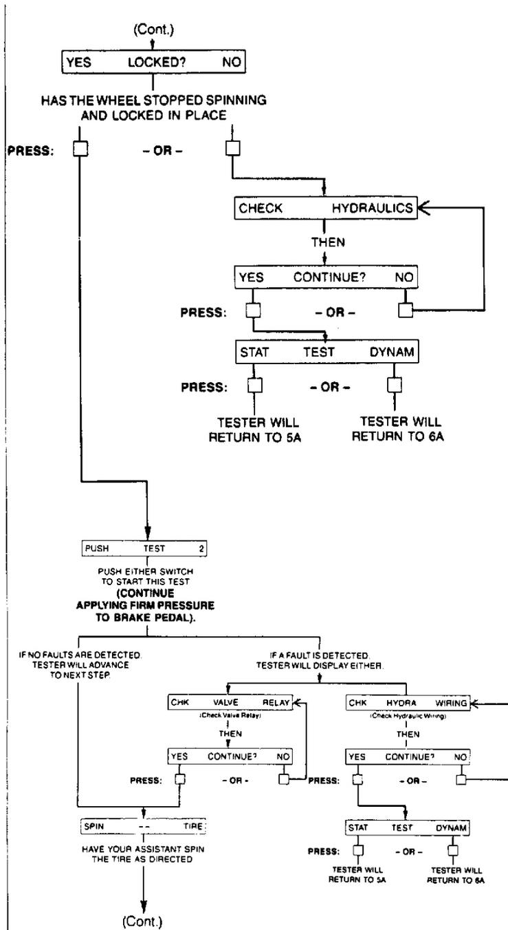
Fig. 25: 6C. Solenoid Test (3 of 4)
