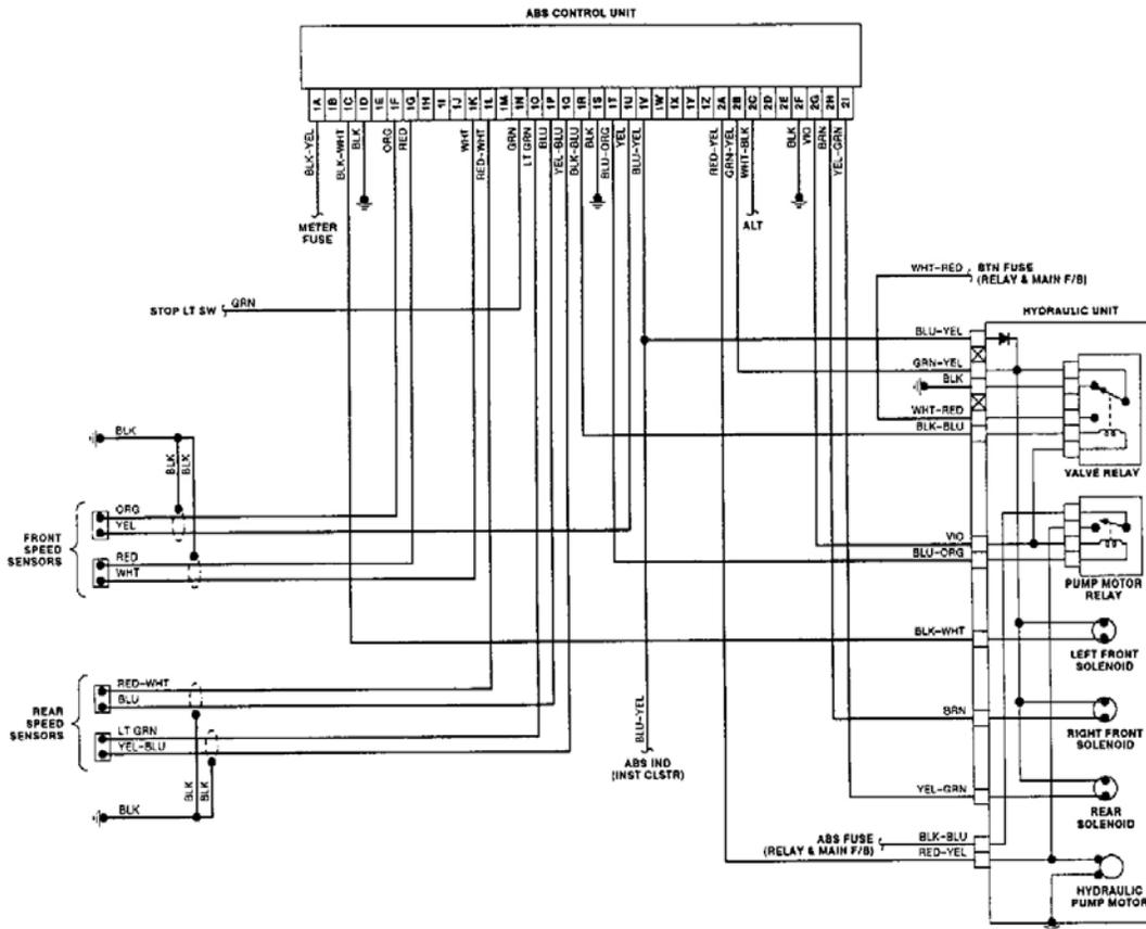
**Fig. 27: Anti-Lock Brake System Wiring Diagram (Miata)**
