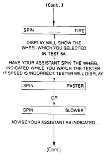
**Fig. 21: 6B. Dynamic Wheel Sensor Test (1 of 2)**
