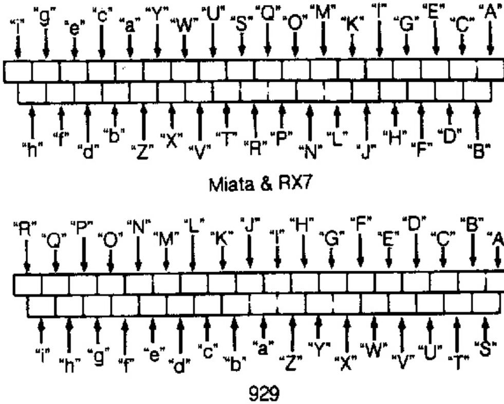
**Fig. 5: Identifying Control Unit Harness Connector Terminals**
