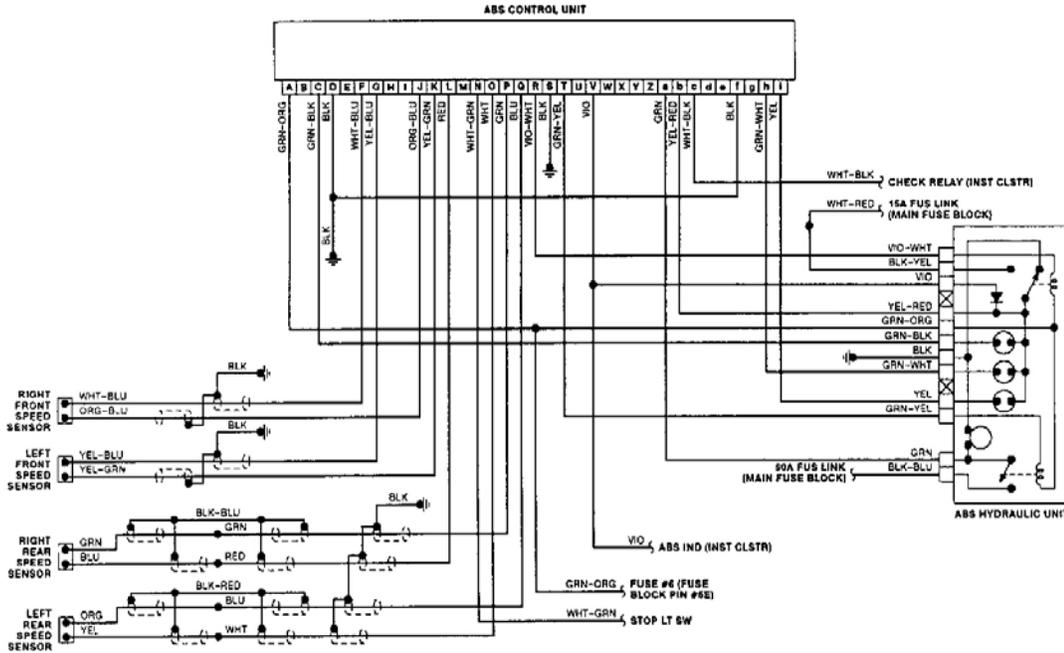
**Fig. 29: Anti-Lock Brake System Wiring Diagram (929)**
