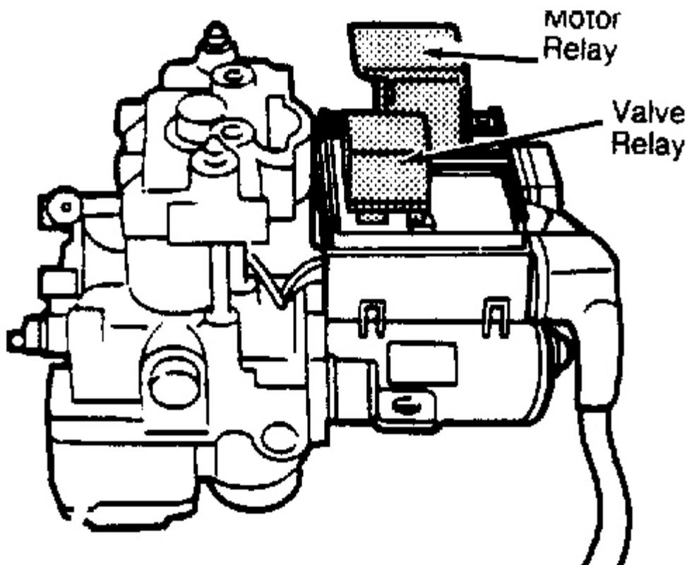
**Fig. 1: Locating Motor Relay & Valve Relay**
