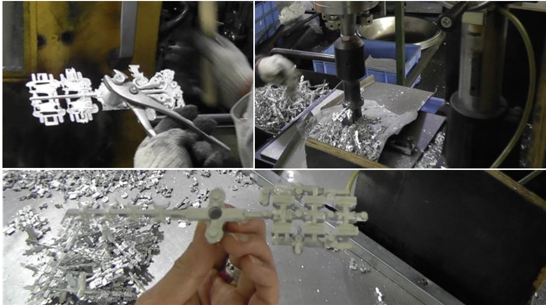
Figure 13, degating, removing the leftover materials.
