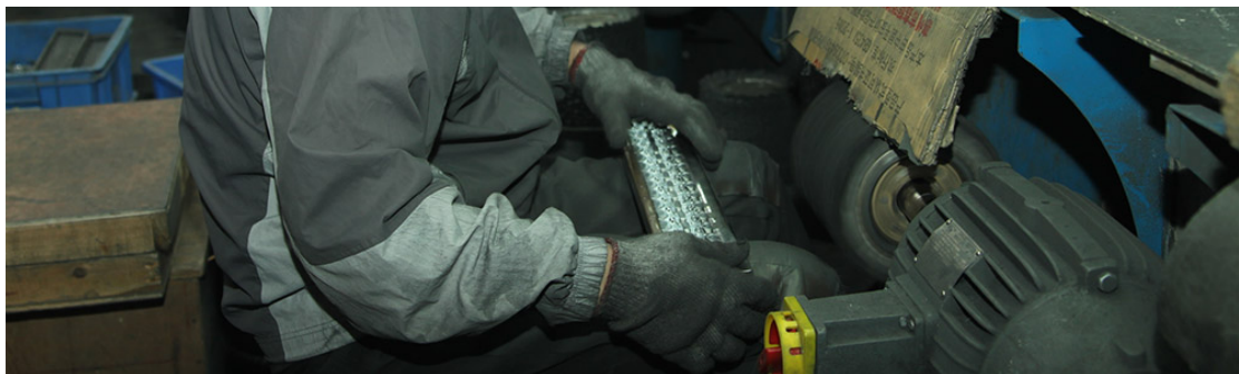
Figure 15, polishing the raw piece to increase smoothness.
