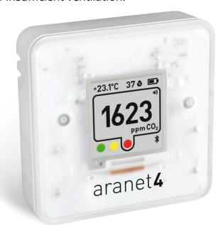
Aranet4 is an easy to use CO<sub>2</sub> monitoring device that lets you know right away if the ventilation is sufficient and whether you are at an elevated risk of SARS-CoV-2 infection via aerosols. Visual color indicators as well as a sound alarm will notify you when action (opening windows, turning up the ventilation or leaving the room all together) must be taken.
