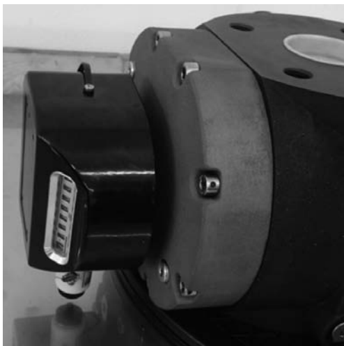
Figure 7: Turning the DN50 index head
