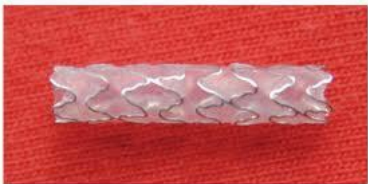
Figure 2. 16 mm-long stainless steel balloon-expandable slotted-tube stent covered with biosynthetic cellulose after drying process.
