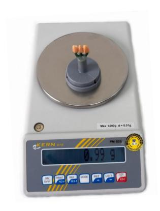
Note: Weight the empty press base - then weigh the press base with the respective modeled object.
