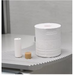
ingot, single-use plunger and muffle
