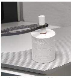
Place the plunger on top of the ingot.
