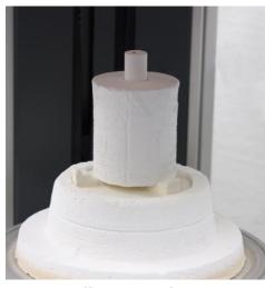
Muffle in pressing furnace
