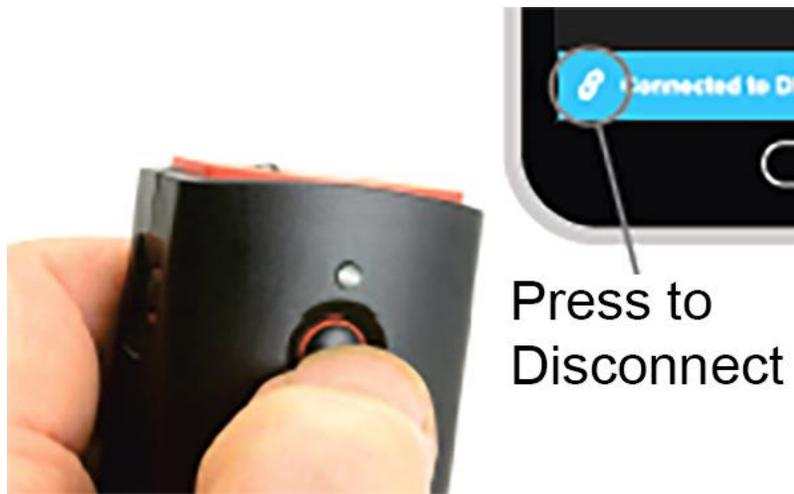
Press the “LINK” icon to disconnect the DMXcat. Press and hold the power button until the LED indicator flashes four times.
