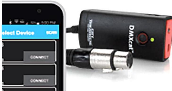
The App connects the smartphone to the device. When the connection is made, the LED indicator will glow steady green, and the lower status bar will display “Connected”.
