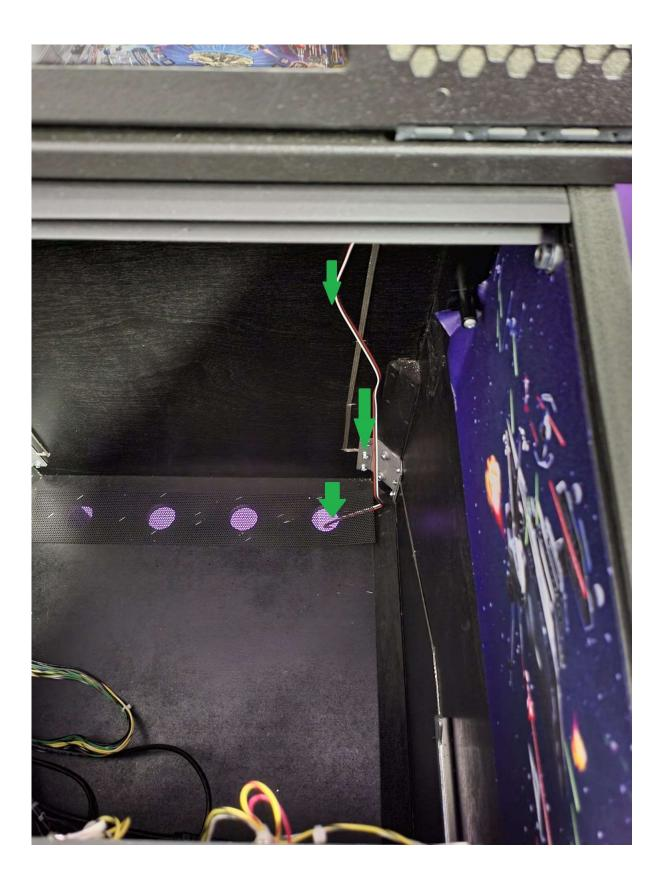
Route the cable labeled CAB-Out downward, and out through the ventilation hole.
