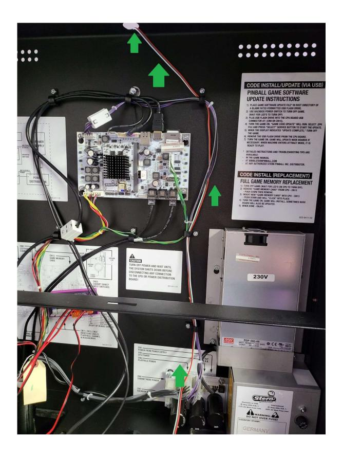
Lay the cable labeled BB-Out in the backbox and lead it out through the upper opening of the backbox.
