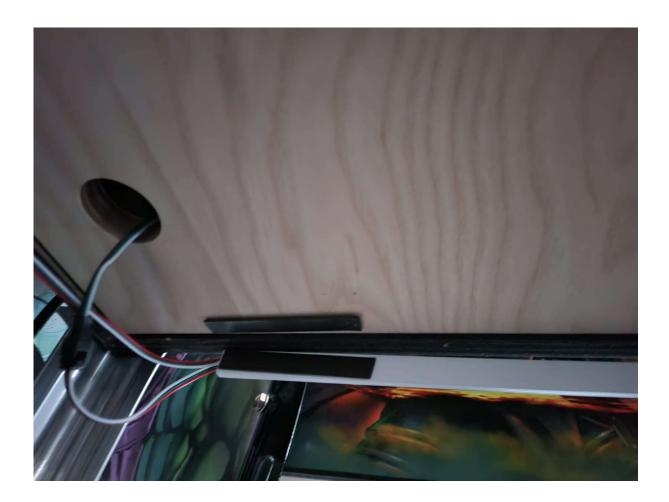
Clean the mounting places for the under-cab lighting under the flipper so that the surface is free of dust or impurities.
