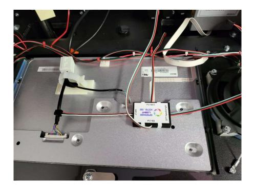
Place the distribution box on the back of the screen. This allows the optional output, the Speakerlights can also be integrated into the system.
