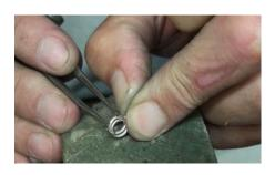
Mark out the four claw points on top of one of the jump rings.
