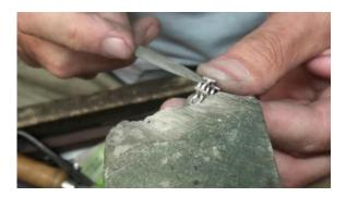
Level off the top of the setting leaving 2mm – 3mm of claw wire for setting the stone.
