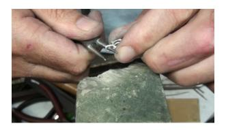
Check to make sure each claw is perfectly square to the setting before quenching and pickling the setting.
