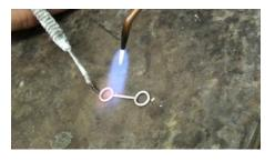
Cut the jump ring coil and close the joints. Make sure the joints are lined up perfectly with no gaps.
