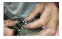
Clamp the bridging wire in the middle with round nose pliers, and carefully bring the two jump rings together.
