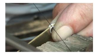
Hold the setting on the spacing metal to prevent movement whilst you perform the cut work. Use a 4/0 blade and cut from the top markings into both rings. Ensure the blade is perfectly square to the setting. Once the marks are cut in, double check with your dividers that the spacing is still positioned correctly.
