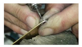
Follow the saw cut with a three square needle file to widen them. Then use a 1mm tapered bur to shape the grooves. Bur approximately a third of the way into the wire thickness. Alternatively you can also use the shaft of a 1mm drill, or a slotting file if you have one.
