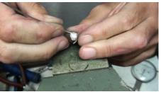
Clamp the end of the wire between your vice and the stake and wrap the wire tightly around, enough to cut two perfect jump rings.
