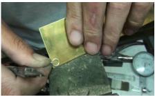
Find a piece of metal sheet or a metal ruler that is approximately 1mm in thickness and tighten the jump rings onto it using parallel pliers.
