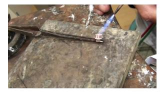
Ensure that the remaining wire is straight, and clean it with 1800 emery paper before cutting four 10mm pieces. This will ensure that the claw wire is free from grease and oxides.
