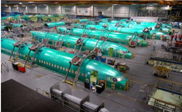
Boeing 737 fuselage in Wichita plant
