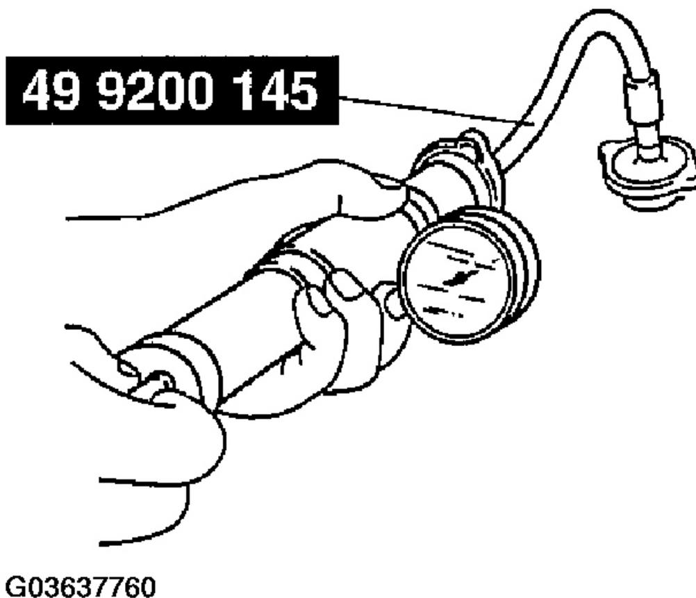
**Fig. 3: Connecting Radiator Cap Tester And SST To Radiator Filler Neck**
