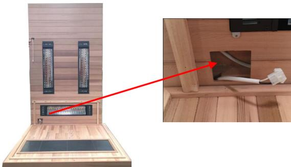
Before place the back panel to the bottom panel, pls pull out the wire of the bottom heater and through the back panel. Then put the back panel onto the bottom panel and make sure its inner side stands against the wooden beam on the bottom panel.
