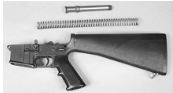
Figure 2-18. Lower Receiver Disassembled.
