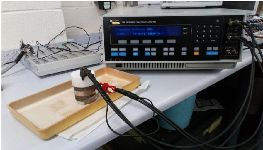
**Figure 20.** Solartron 1260 Impedance analyser with coaxial sealant sample.
