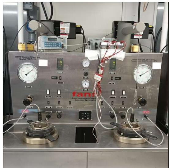
**Fig. 3.** Autoclave/logging system during curing process.
