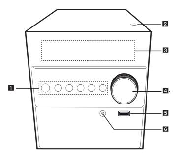
1 U/ (Standby/On) 2 △ (Open) Switches the unit ON or OFF. 3 Display window F (Function) Selects the function or input source. 4 Volume Knob **I**≪/≫ (Skip/Search) Adjusts volume of speaker. - Searches backward or forward. 5 USB - Skips to the previous/next track/file. TUNING - / + device. - Selects the radio stations. 6 PORT. (Portable) IN - Scans DAB+ stations by pressing and holding. Connects to a Portable device.
