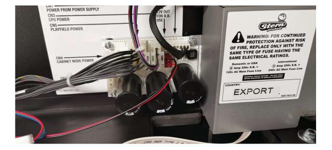
Place the voltage transformer (small black box) in the backbox and close the cover.
