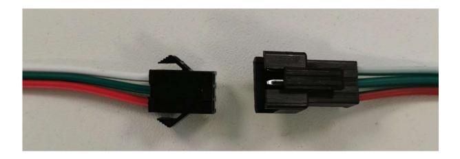
When mounting the connector on the board, make sure that + and - are not interchanged.
