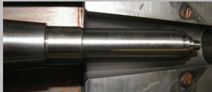
Coated tool by ALLWIN, Cr-Al-Si based coating Thickness: 2 to 3 μm
