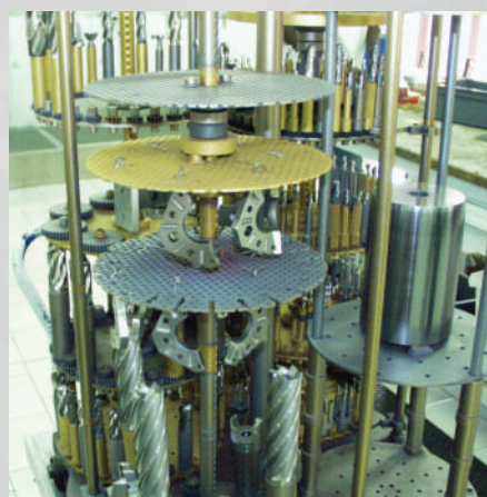
Large volume job coating load with different mixed substrates
