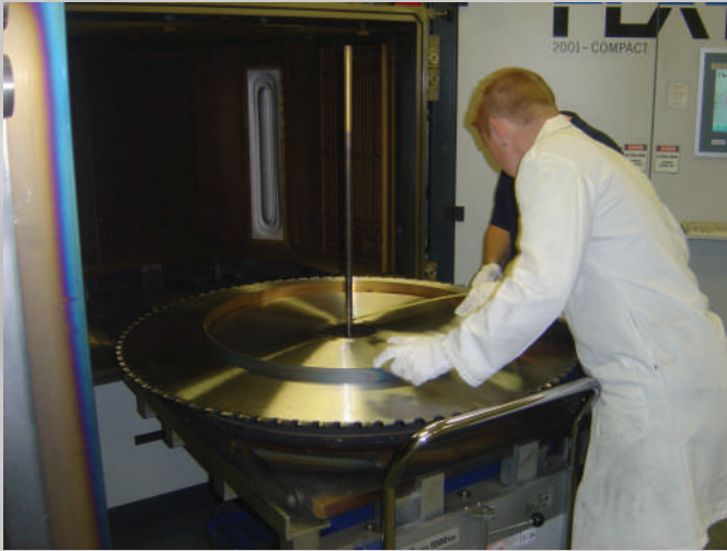
Setting the distance holder for big saw blades before coating
